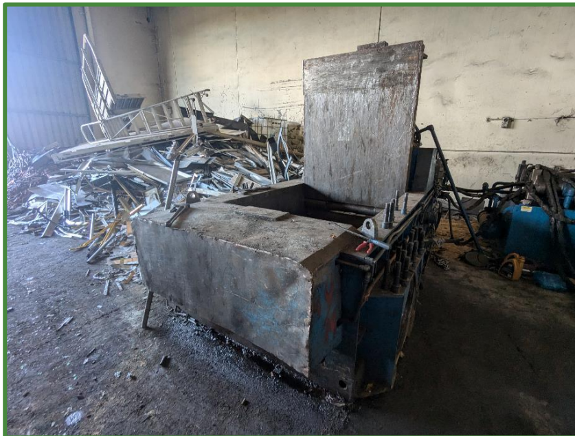
Photograph 31: Metal baler within metalworks building (not operational during visit). Note probable loss of hydraulic oil beneath the baler. An aluminium stockpile is visible in background. Hydraulic pump is visible to the right. Sand across floor visible along western wall of building (viewer facing southwest).
